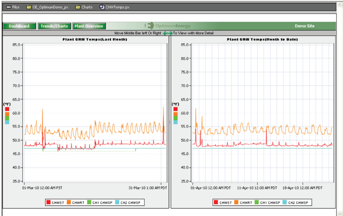
Figure 8: The OptimumMVM Chilled Water Trend Chart is one of a dozen pre-defined views.
